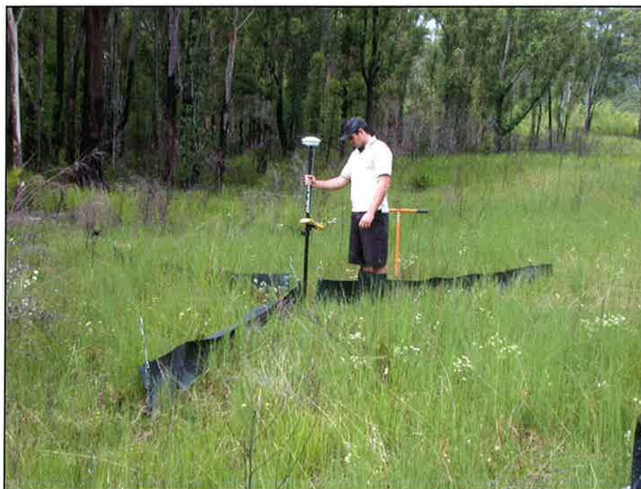
Photo 5. Pitfall trap with three drift fences set out at an angle of 120°. Locating pitfall traps using high-powered GPS.
